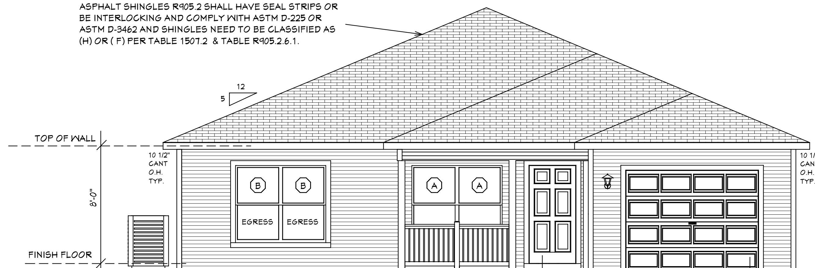
FRONT ELEVATION TOP OF GARAGE DOOR AT 7'0" TALL U.N.O. DECORATIVE NON-STRUCTURAL RAILING TOP OF ALL WINDOWS AND DOORS AT 6'-8" A.F.F. U.N.O. HORIZONTAL VINYL SIDING (TYPICAL AT ALL ELEVATIONS)
